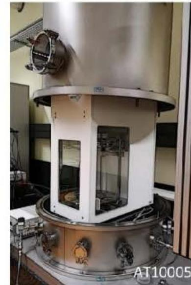
Figure 1: Mass comparators in air-tight enclosures in METAS
