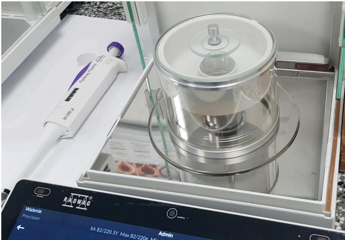
Fig. 12. XA 82/220.5Y balance with a 17-ml weighing vessel.
