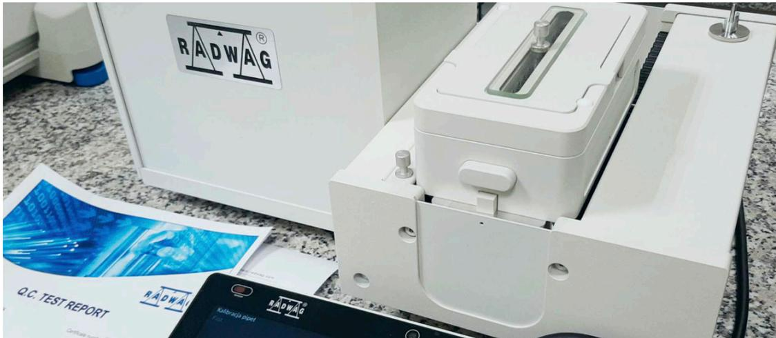
Fig. 18. AP 12.5Y automatic unit during metrological check
