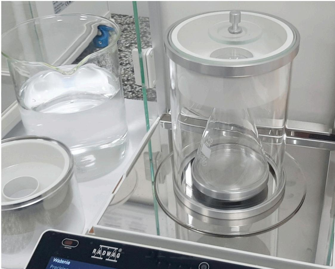
Fig. 15. XA 82/220.5Y with a 100-ml weighing vessel
