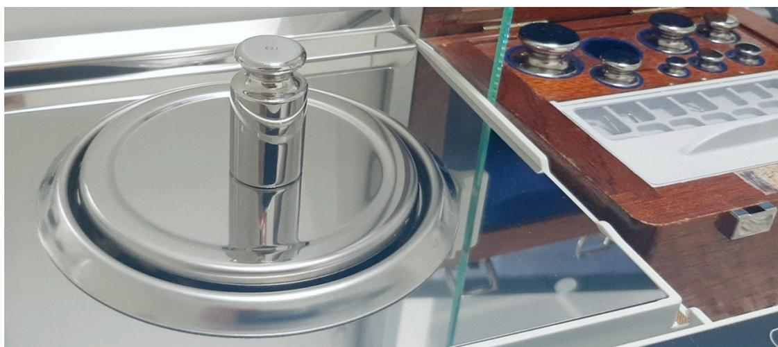
Fig. 4. Balance stability control with mass standard
