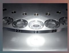
Special light system inside the chamber facilitates precise loading of mass standards and helps to find and remove potential impurities.
