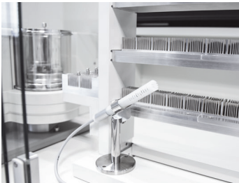
The mass comparator allows real-time monitoring of ambient conditions.
