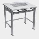
The antivibration table has been designed to eliminate floor vibrations during the operation of industrial scales. It consists of two separate constructions: the outer, designed to isolate the working part, and the inner. The working part includes a table and a stone separated by a vibration damper. The table features a large stone top and adjustable feet with protective rubber tips, facilitating table levelling on uneven surfaces.
