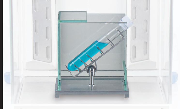
The holders have the ability to tilt the microscale glassware, allowing it to be placed at any angle, depending on the application. The set includes dedicated draft shields that stabilize the measurement conditions in the weighing chamber.
