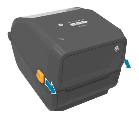
Slide the release latches to the front to unlock the cover.
