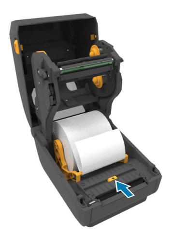
Align the sensor to the center of the roll for regular labels.
