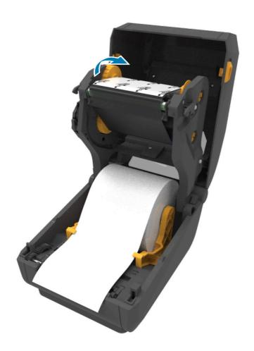
Turn the ribbon take-up wheel to remove the slack and advance the ribbon.
