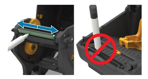
Clean printhead with cleaning pen starting from the middle to sliding to the outside. Do not use a cleaning pen on the platen.
