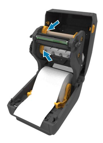
Place the left side of the spool onto the spindle aligning it with the notches.
