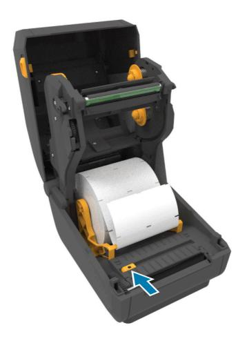
Align the sensor to the edge of the roll for marked labels.
