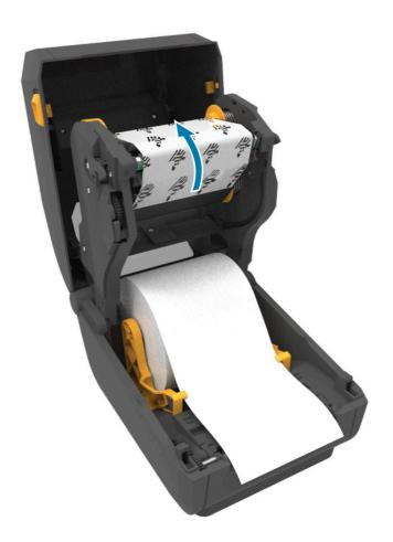
Pull the supply ribbon leader up and over the printhead and attach it to the take-up spool.
