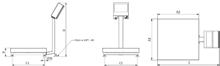
Scales of WPT...H1 series (extension arm 7cm)
