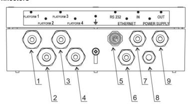
MW-04 mass converter connectors
