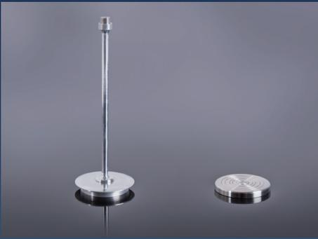
Weighing pans construction facilitates their easy replacement and quick switching between susceptometer, microbalance and mass comparator.
