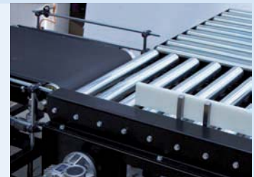
Line with belt conveyors and roller conveyors with a pneumatic rejecter
