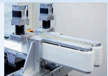
Vertical, flexible system of side guides used for transporting bottles
