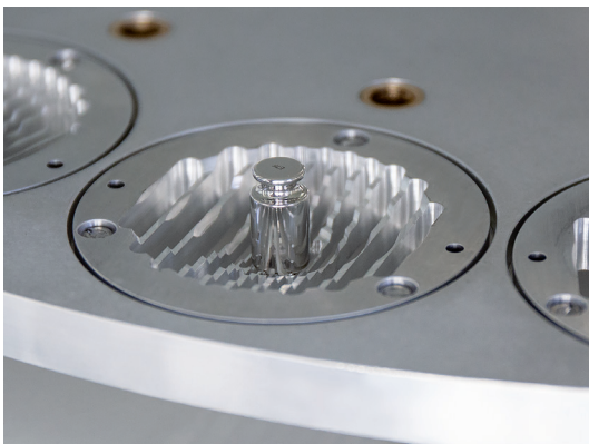
Universal insert for UMA-1000 guarantees precise measurement of 10 g - 1 kg mass standards regardless of shape and size.
