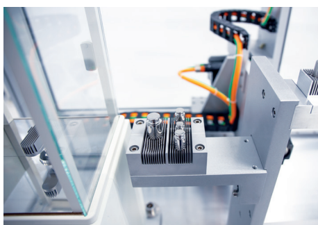
Intermediate mass standard magazine significantly shortens calibration and facilitates dissemination.
