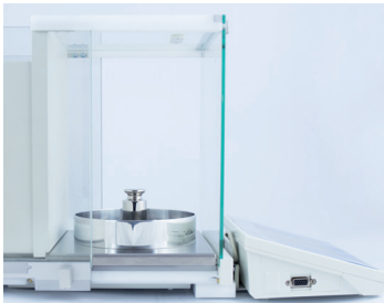
Spacious and airtight weighing chamber of XA 4Y.A.KB mass comparator features automatically opened door.
