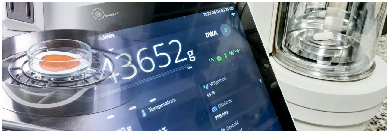
Figure 11. XA 82/220.5Y balance, filter mass measurement, MYA 2.5Y microbalance, capsule mass measurement - uniformity of medical preparation mass (USP)
