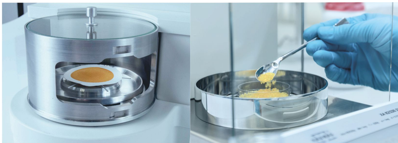
Figure 8. Testing filter mass changes after filtration, measuring the amount of substance
