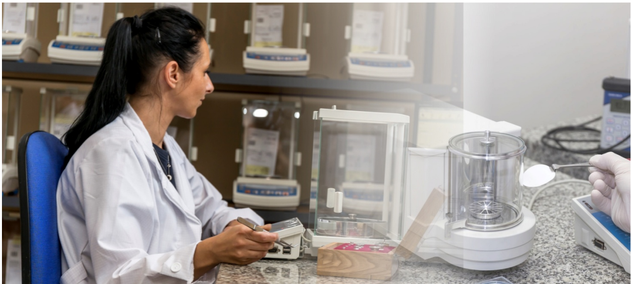
Figure 13. Balance metrological inspection, filter mass measurement
