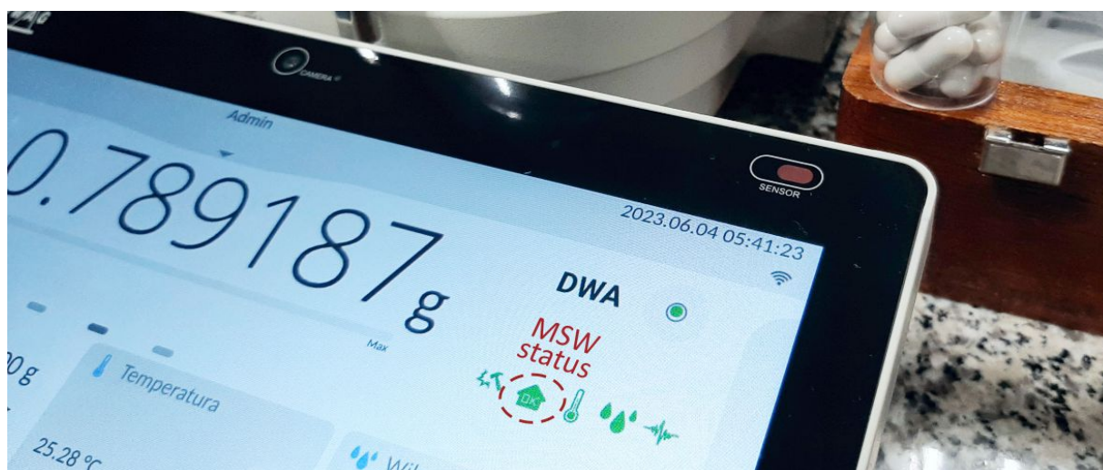
Figure 9. MYA 5.5Y microbalance with an active MSW function
