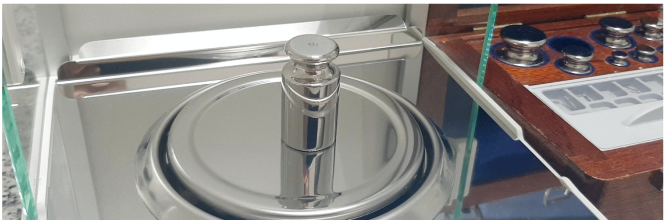
Figure 6. Balance sensitivity deviation control using a mass standard
