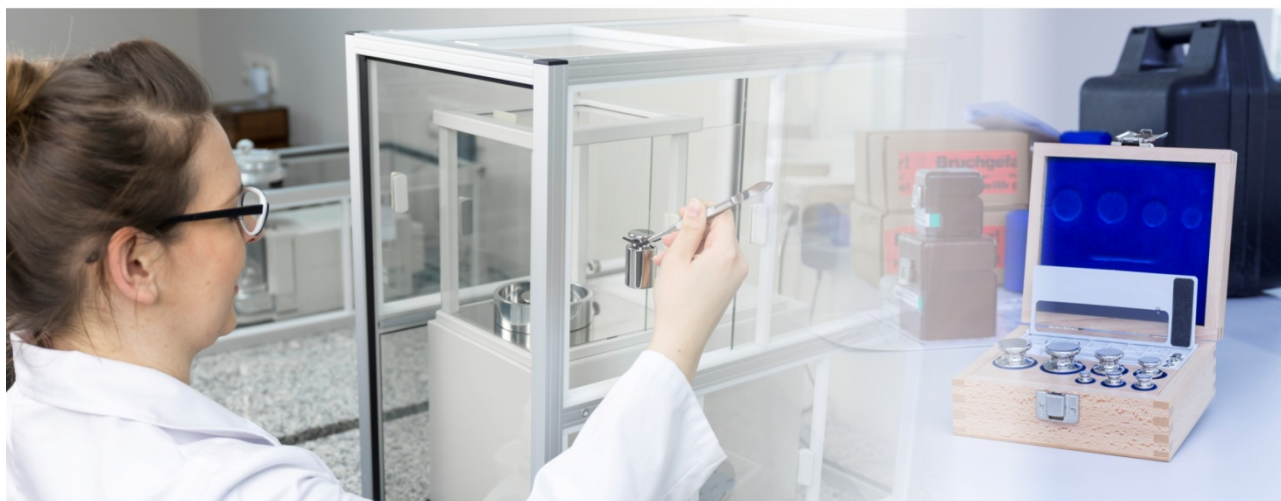
Figure 2. Mass comparator calibration using manual method
