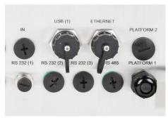
The back side of the housing features hermetic connectors of communication interfaces.
