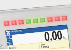
The bar graph, consisting of 9 red and green diode fields, is located at the top of the operation panel, it visualises a current net weight value.
