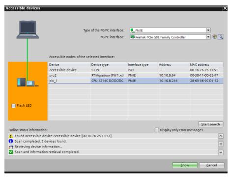
Now, specify the module IP address and its name in the PROFINET network. After selecting the module in the PROPERTIES tab, find the PROFINET INTERFACE submenu and enter the IP address and a name. Make sure that the setting is accordant with the parameters set in the scale menu. Make sure that IP SLAVE address is in the same subnet as the MASTER address.
