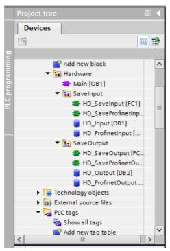
HD\_OUTPUT and HD\_INPUT blocks represent physical input/output registers of the MASTER controller and are not relevant in this project. HD\_ProfinetOutput and HD\_ProfinetInput blocks represent input/output registers of the scale's PROFINET module. See the screenshots below:
