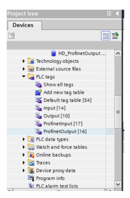
INPUT and OUTPUT tables refer to physical inputs/outputs of the MASTER controller and are not relevant in this application. ProfinetInput and ProfinetOutput blocks represent input/output registers of the scale's PROFINET module. See the screenshots below (names and addresses are examples only):
