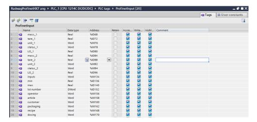
In order not to operate using module's physical inputs/outputs create data blocks containing representations of these registers and functions rewriting values between them. Create HARDWARE group in the PROGRAM BLOCKS branch and determine data blocks as below:
