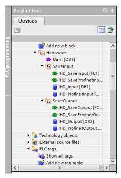
HD OUTPUT HD INPUT blocks physical MASTER's and refer to inputs/outputs and are of no importance in case of this project. HD ProfinetOutput and HD\_ProfinetInput blocks represent input/output registers of the scale's PROFINET module. See the screenshots below:
