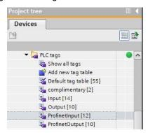
INPUT and OUTPUT tables refer to physical inputs/outputs of MASTER controller and are of no importance in case of this application. Input and output registers of PROFINET module have been specified in ProfinetInput and ProfinetOutput tables.
