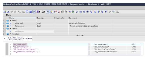
Upon compilation and upload of the program to the controller in data block it is possible to read input registers (MONITOR ALL) and to record output registers (e.g. by change of START VALUE and LOAD START VALUES AS ACTUAL) of the SLAVE module.
