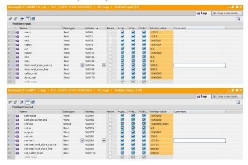
So as not to work directly on the physical inputs/outputs of the module it is recommended to create data blocks comprising representations of these registers, and functions "copying" values between them. For this purpose HARDWARE group is created in the PROGRAM BLOCKS directory, the blocks are defined as below:
