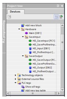
HD\_OUTPUT and HD\_INPUT blocks refer to physical MASTER's inputs/outputs and are of no importance in case of this project. HD\_ProfinetOutput and HD\_ProfinetInput blocks represent input/output registers of the scale's PROFINET module. See the screenshots below:
