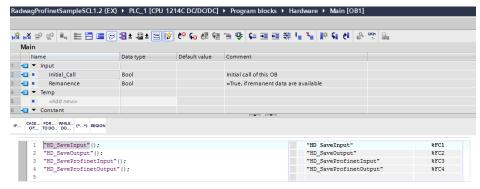
Upon compilation and upload of the program to the controller, in data block it is possible to read input registers (MONITOR ALL) and to record output registers (e.g. by change of START VALUE and LOAD START VALUES AS ACTUAL) of the SLAVE module.
