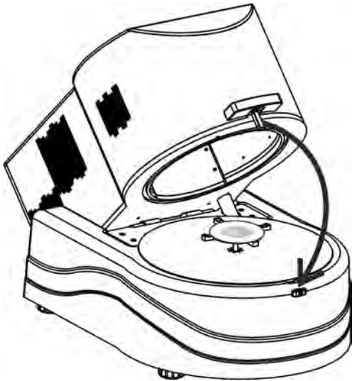
The drying process is started automatically. The moisture analyzer starts drying process according to pre-set parameters and the display indicates data on carried out process. During the drying process the moisture analyzer carries out all necessary mass measurements and calculations resulting from mass change, and sends a header to a specific communication port (compatible with settings of printout options).
