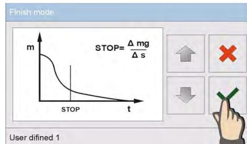
The previous window is displayed. Displayed data refer to selected finish mode. Set parameters to operator needs by pressing a name of data to be edited.
