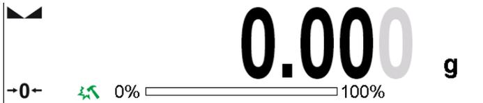
If incorrectly carried out loading is detected, the pictogram turns to red
