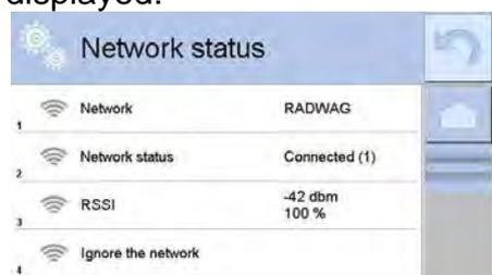
The selected network and connection parameters are saved to moisture analyzer memory. The program connects to the network in accordance with the memory-saved parameters each time the moisture analyzer is switched on. To change this, select <Ignore the network> entry. Given network gets disconnected.
