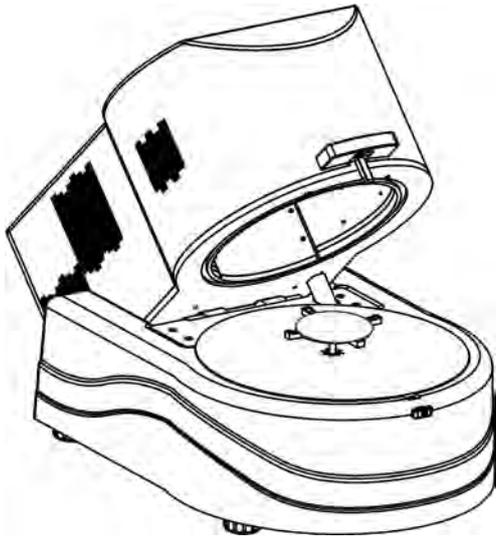
Weighing pan mass is displayed. It is recommended to close the drying chamber in order to provide stable ambient conditions while taring.
