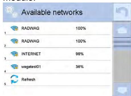
Pictogram with a padlock means that the password is required. Press <Refresh> pictogram to search for available networks.
