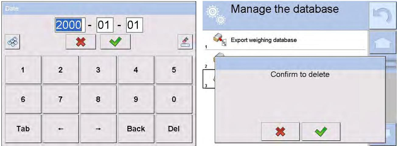
Confirm the date, all weighings and reports older than those specified by the date are removed. Quantity of deleted weighings and reports is displayed.
