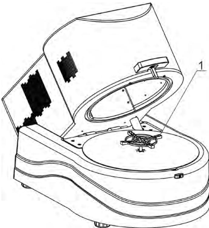
1. Cross-shaped holder on which filters with sample are placed.
