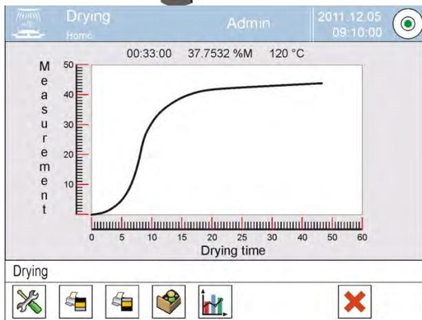
Drying graph containing data regarding the process is displayed. The graph is created in real time. This enables monitoring the process in actual time. To monitor the graph for various units, determine humidity unit prior to displaying the graph. Next, enter the graph.
