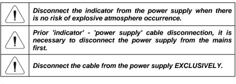
Cable disconnection procedure:
