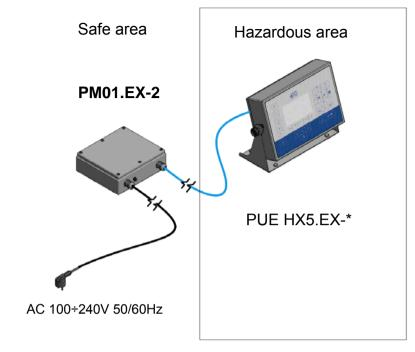
Fig .3. Power supply in safe area
