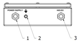
Fig.6. Power supply connectors arrangement PM01.EX-\*
