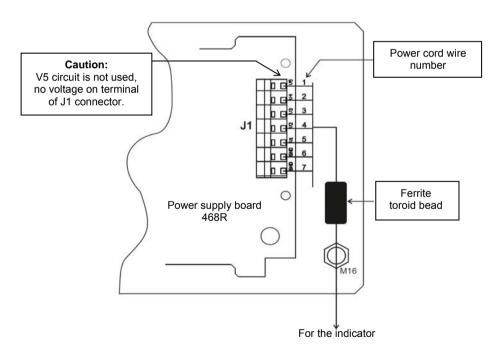
Fig.7. Connection method of the intrinsically safe cable
