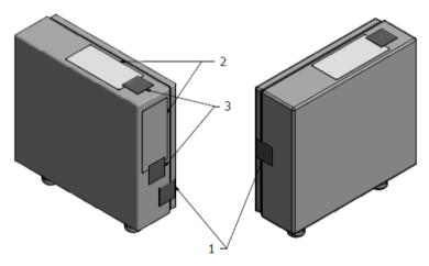
Fig.5. Arrangement of data plates and security stickers
