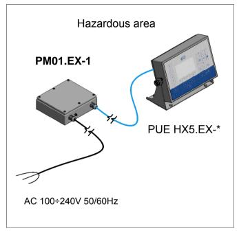
Fig.2. Power supply in hazardous area
