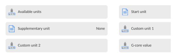
Here, it is also possible to enter the gravitational acceleration value in the place of using the balance. It is required for using the mass value in [N].
