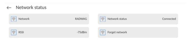
The selected network and connection parameters are remembered by the balance program. Every time you turn the balance on, the program connects to the network as per your preset parameters. To disable this function, select <Forget network> item. It will cause the connection to the specific network to be terminated.
