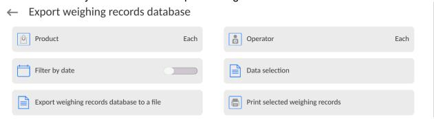
In <Data selection> field, the operator can define data related to measurements to be exported.
