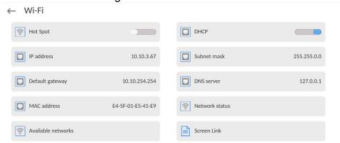
2. Activate the Hot Spot service and the balance will switch into service settings after a while.
