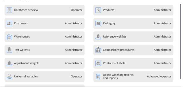
Default balance settings allow the operator logged as an **Administrator** to make changes to settings of particular databases. Depending on requirements, these permission levels can be changed.
