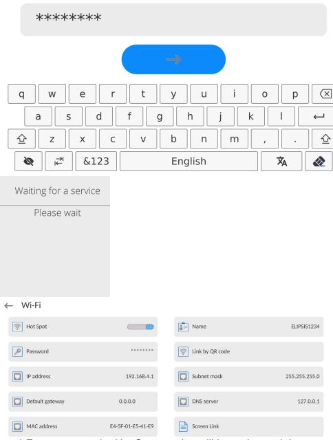
4.From now on, the Hot Spot service will be active and the created subnetwork will be recognised by other devices, such as a smartphone, under the aforesaid name, and it will be possible to connect to it with the password.
