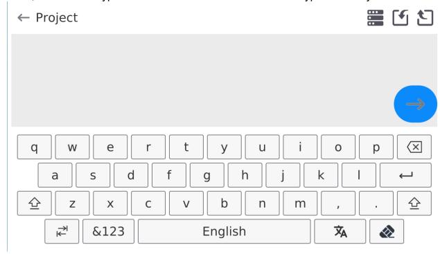
The displayed keypad does not provide some characters and signs, such as colon or diacritical signs typical of a language (menu language is signalled with the 'SPACE' key description). To use such signs in the printout designed, **press and hold** a specific letter on the keyboard for a while. This will cause additional keys with assigned signs to be displayed. You can click them to add a text. After you have entered the sign, disable the signs by pressing the 'X' key.
