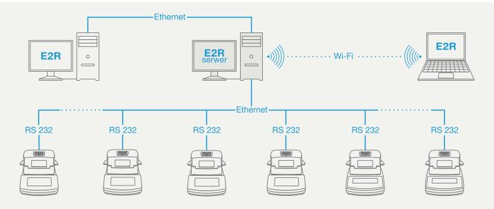
Software functions: on-line monitoring of moisture analyzer operation, possibility of configuring reports and graphs, analysis of data collected from many drying workstations, data protection.
