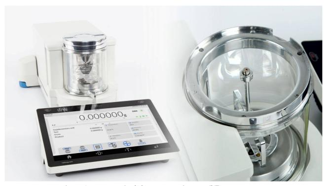
**Figure 43. MYA 5.5Y microbalance – magnetic susceptibility measurement**MYA 5.5Y microbalance, maximum load 5g, elementary reading unit d=0.001mg, OIML certificate
