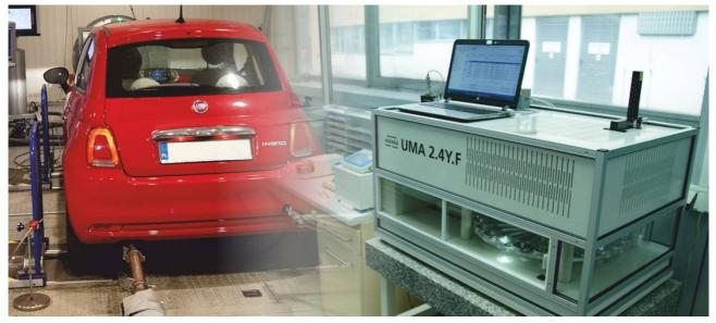
Figure 30. Chassis dynamometer and filter mass measurement automatic unit.
