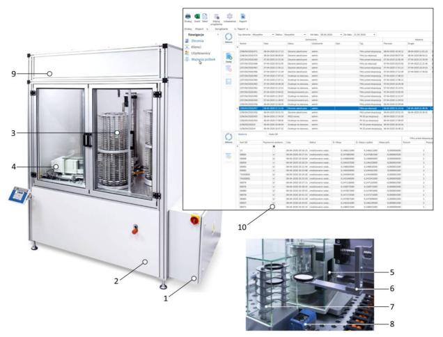
Figure 29. RB 2.5Y – filter conditioning and mass measurement
