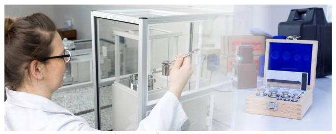
Figure 5. Manual WAY mass comparator
