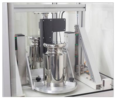
Figure 2. AKM comparator 2.20.5Y,d= 0,1 mg
