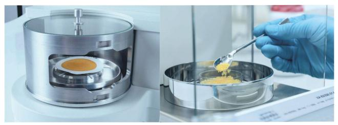
Figure 13. Testing changes to filter mass after filtering (wastewater treatment plant), measuring the amount of substance (pharmacy)
