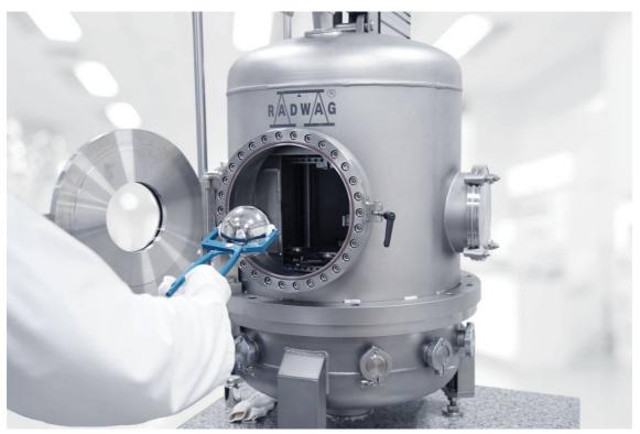
Figure 3. AVK 1000.5Y vacuum comparator
