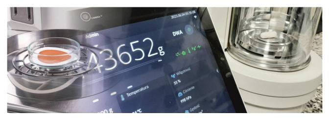
Figure 22. XA 82/220.5Y balance, filter mass measurement,
