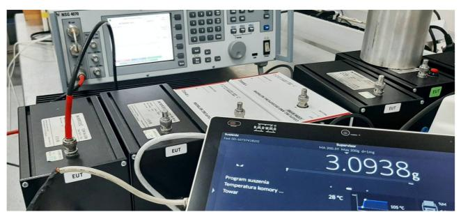
Figure 49. Testing the electromagnetic compatibility of the balance with 5Y terminal Test: resistance to radio signals
