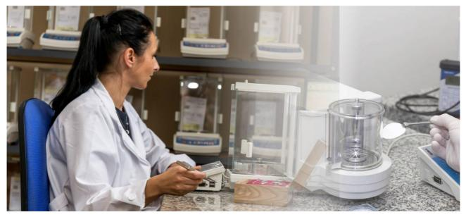
Figure 53. Non-automatic balance metrological verification
