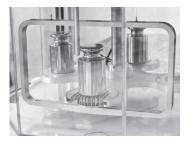
The weighing pan suspended on wires with a diameter of 0.3 mm allows minimising non-centricity errors and eliminates the impact of surface tension of the liquid.
