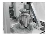
2-position magazine for 1 reference standard and 1 test standard.
