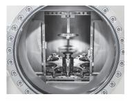
Self-centring suspended weighing pan elimination of a non-centricity error thanks to the use of a special suspended weighing pan.
