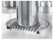
Thanks to a special structure of the insert, the comparator offers a wide measuring range (from 1 g to 1 kg) and is adapted to comparing silica hemispheres.
