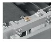
The programme guides the user through the process of checking the magnetic properties of the test sample and automatically changes the magnet's polarity at the appropriate time.
