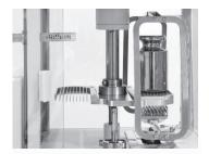
Elimination of a ecentricity error thanks to the use of a special suspended weighing pan.
