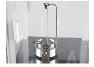
Weighing pan, made of the best quality non-magnetic stainless steel, features centrically positioned markings allowing easy and precise weights placement.
