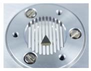
Comparison can be carried out for weights of all shapes with use of just one universal weighing pan.
