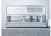
Compact size guarantees operation of the device at any laboratory workstation. Possibility of comparison of many weights at a time adds to comparator's versatility.
