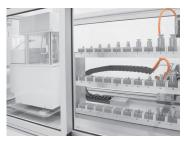
Combination of advantages of the robotic system and automatic system. A few-time better repeatability in view of stable ambient conditions during comparison due to the fact that the weighing chamber does not open throughout the cycle.
