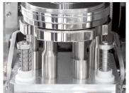
Fully automated change of the comparison range in comparators equipped with inner ballasts.
