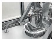
The automatic mass loader (loading robot) features a basis with self-centering fields, lift and weighing module equipped with a selfcentering pan.
