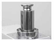
Ring-shaped draft shield encircling the weighing pan, apart from protecting the pan against air drafts, prevents potential shocks that could be applied accidentally to the weighing pan while loading the weight.
