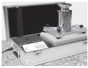
Dedicated box for PM 5Y.KB mass comparator is a warranty for safe transport. With in-built interfaces you have a green light for immediate operation right after opening the box.
