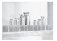
The mass standard magazine offers up to 100 magazine positions, this number is conditioned by a comparator model. the device enables comparison of weights of all shapes compliant with OIML recommendations, using just one universal insert.
