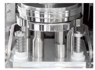
Fully automated change of the comparison range in comparators equipped with inner ballasts.
