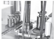
The mass comparator enables a complete dissemination process, which is possible due to placing the intermediate mass standard magazine inside the mass comparator chamber. This significantly shortens comparison duration and reduces wear and tear of the transport robot.
