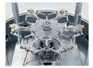
6-position mass standard magazine for calibration of cylindrical standards ø(22-95)x110 and silicon spheres with a diameter from 40 to 100 mm
