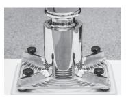
Centering holders of the openwork weighing pan allow precise placement of the weights, it is especially helpful when working with heavy and large mass standards.
