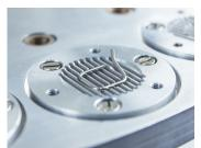
The weighing pan has been designed to enable measurement of very small samples with very high precision. This also secures a weight against wedging.
