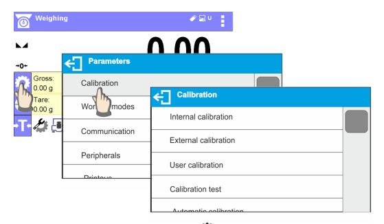
In order to enter moisture analyzer menu press PARAMETERS> entry. Pressing any button comprised within workspace or pressing parameter name results with change of colour. If a given area has any function or action assigned, then it is performed automatically upon pressing (e.g. adjustment procedure), respectively a particular window with parameters or a list of appropriate settings is displayed.
