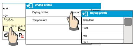
Enter drying profile settings and select respective drying profile. Upon selecting a profile, set its respective parameters. Parameters depend on selected profile.
