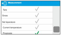
5. On setting the above parameters you can start drying process by following the above description. On starting the drying process an additional button is displayed in the bottom part of the display. On pressing this button, a window with prognosis is displayed. In the initial stage of the drying process there is no result of prognosis yet and the <Calculating> status is displayed in the prognosis window.
