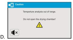
E. Follow the displayed prompt. Wait until the temperature decreases to a safe level, which is signalled by a new prompt.
