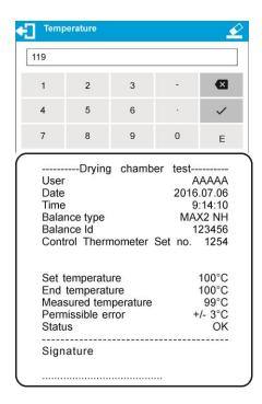
The temperature is maintained for 8 minutes (like for temperature adjustment procedure). After 8 minutes you shall see a window for entering temperature read from the installed adjustment set.
