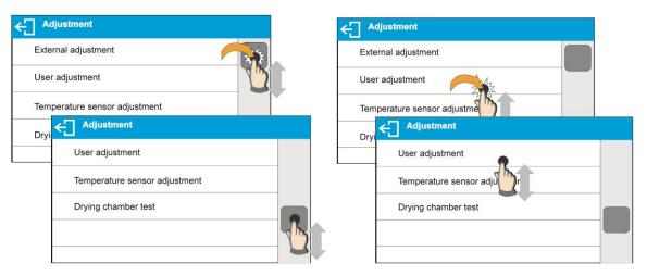
There are two methods for scrolling the screen of parameters window. The first one requires pressing, holding down and scrolling up or down the scrollbar located on the right. The second one requires pressing, holding down and scrolling up or down any point of the displayed window.
