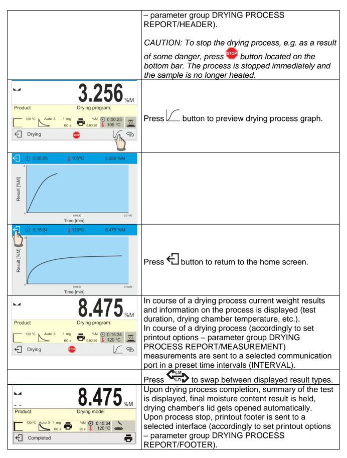
Drying process can be aborted at any time. Press button to abort the drying process and press button to confirm.
