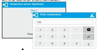
Press button to confirm, the third step of adjustment starts. The moisture analyzer halogen lamp starts to operate and the drying chamber is heated as long as necessary to provide specified temperature, which is next maintained for 8 minutes. After 8 minutes a numeric keyboard is displayed. Enter the moisture analyzer temperature that is displayed on the control thermometer.
