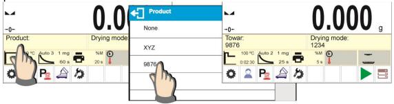
5.Additionally, when choosing the product, you can use the BIAS function. This function allows you to adjust the drying result automatically and display the adjusted valued in the information field while drying.
