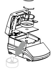
When installing the weighing pan cross, pay special attention to location of a cross mandrel.
