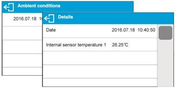
Caution: The software saves ambient conditions record in a so called loop, i.e. when the measurement 10 001 is saved, the measurement 1 gets automatically deleted from the moisture analyzer memory.
