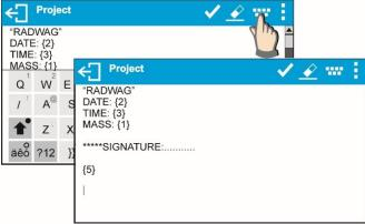
In order to carry out HEADER or GLP or FOOTER printout using EPSON printer (equipped with an auto-cutter blade) and crop the paper beneath the respective printout, select an option of non-standard printout comprising {150} variable, and set this option in header, GLP printout or footer settings, respectively. (For instruction on how to enter control codes, read section 21 of this user manual).
