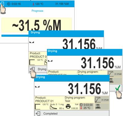
8. On drying process completion a footer of drying report containing status, end result and estimated result are printed. The estimated result is a result that would be achieved on reaching the criteria set by the user for a given process.
