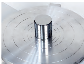
Positioners on the susceptometer weighing pan facilitate centring of the mass standard.
