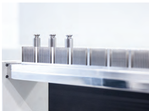
The mass standard magazine offers up to 120 magazine positions.
