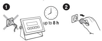
Prior to switching the device on let it reach room temperature (estimated stabilization time: 8 hours).
