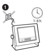
Prior to switching the device on let it reach room temperature (estimated stabilization time: 8 hours).
