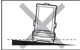
Make sure that the balance is placed on an even surface.
