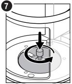
Install and tighten the protective ring using the handle.
