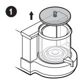
Lift the lid of microbalance weighing chamber.
