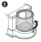
Open the weighing chamber by twisting the handle.
