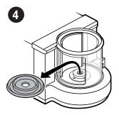
Remove the draft shield from the weighing chamber.
