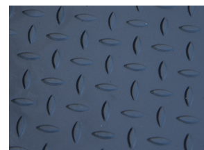
The upper part of the weighing pan is a tear plate surface
