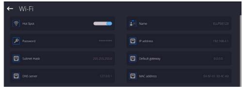
4. From now on, the Hot Spot service will be active and the created subnetwork will be visible by other smartphone devices under the name assigned above and you will be able to connect to it using the assigned password.
