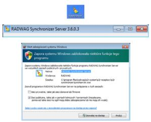
If Windows OS system has **Windows Firewall** set to active, it should switched off before the first run of the software.
