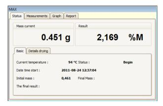
If a specific moisture analyzer does not communicate with **Radwag Synchronizer** service, then a window with current mass display indicates
