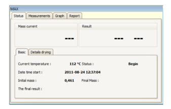
If a window of current measurement result indicates "---" characters, it means that a moisture analyzer lost communication with **E2R Manager** or on after connecting no measurement were recorded.
