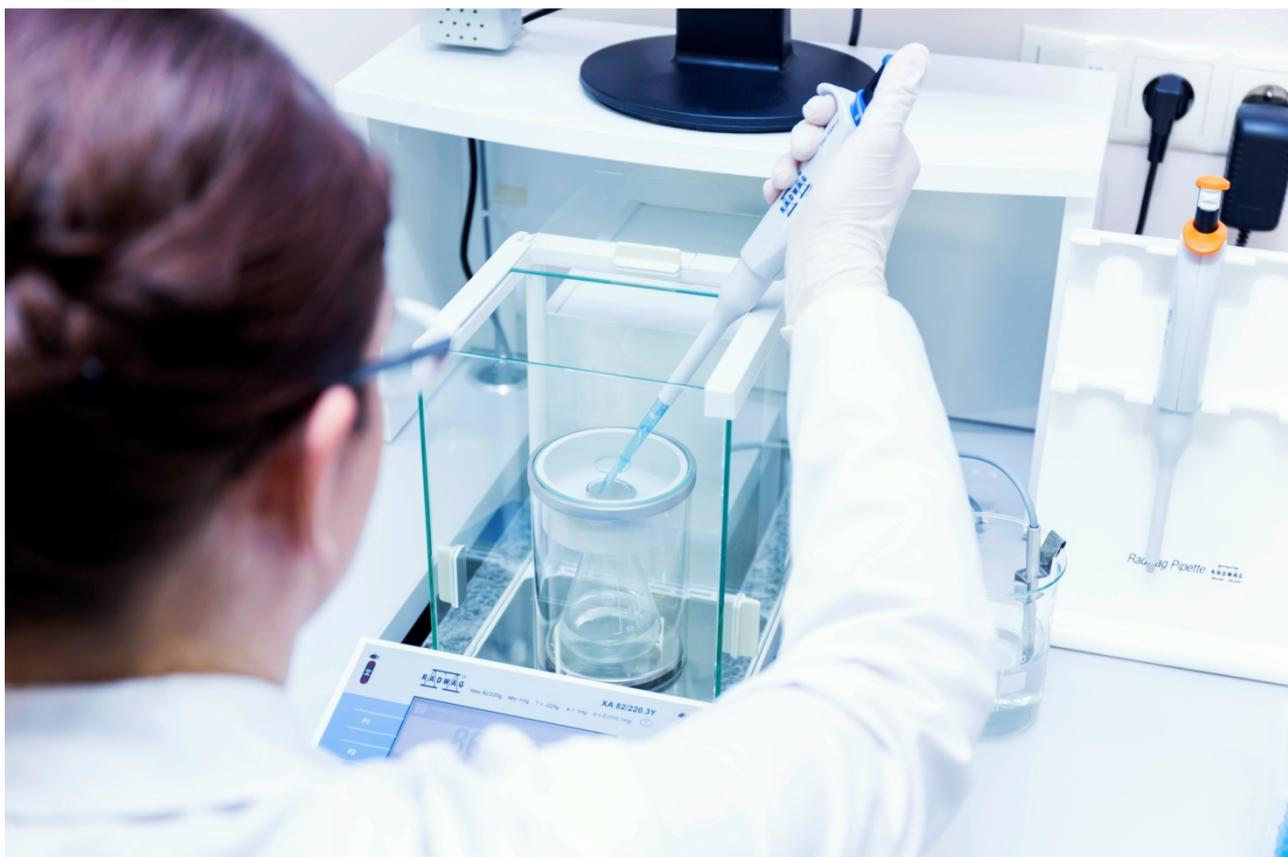
Photo 6. Inspecting piston pipette (200  $\mu$ l of volume)
