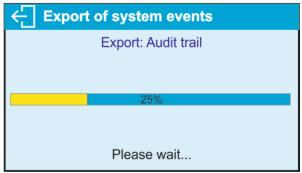
When the process is complete, the window is closed and the data is saved to the USB flash drive in the file: "AuditTrail 589523 2022 02 08 12 15 15.txt."
