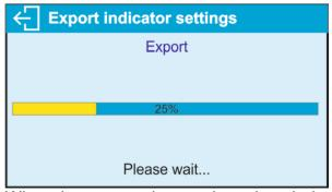
When the process is complete, the window closes and the file is saved on the USB flash drive as: "update589523\_220208\_1227.x3prg" – file with balance settings, "Backup589523\_220208\_1227.x3cfg" – file with balance data.
