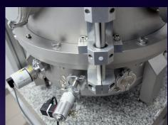
The main chamber of mass comparator is equipped with 8 flanges (DN 40 ISO KF) for connecting devices such as vacuum gauge, solenoid valves, CO2 sensors etc. LOAD LOCK chamber features 2 such flanges.
