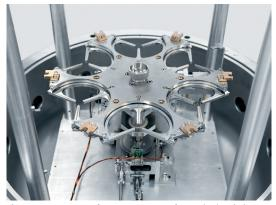
The mass comparator features magazine for 6 cylindrical objects of  $\emptyset$  (22 - 95) x 110 mm or sphere objects of maximum diameter of  $\emptyset$  100 mm.
