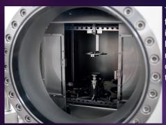
The mass comparator features second, integrated weighing pan. It is used to compensate mass during calibration of mass standards lighter than 1 kg.
