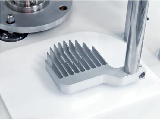
The comparator features specially designed feeder to load and unload the magazine with mass standards.
