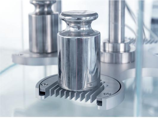
Special design of the insert ensures very high measuring range of the comparator (1g-1kg or 1kg-20kg). It is also intended for comparison of silicone spheres.
