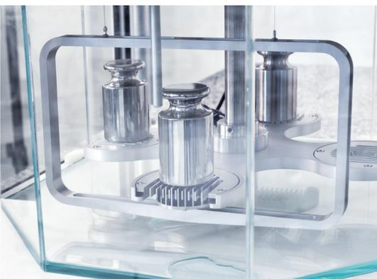
A weighing pan suspended on wires of 0.3 mm diameter significantly minimizes the eccentricity and eliminates the influence of liquid surface tension.
