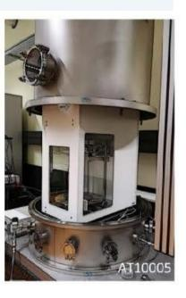
Figure 1: Mass comparators in air-tight enclosures in METAS
