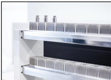
**The mass standard magazine offers up to 120 magazine positions,** this number is conditioned by a comparator model. The device enables comparison of weights of all shapes compliant with OIML recommendations, using just one universal insert.
