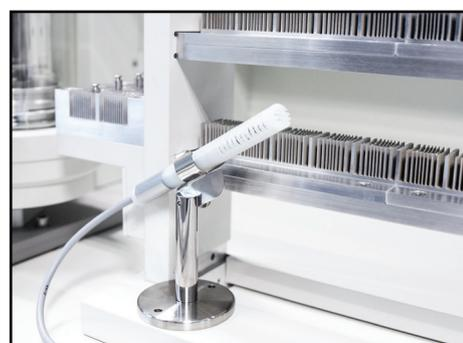
The mass comparator allows real-time monitoring of ambient conditions in three different locations with a very high accuracy: pressure with the readability of 0.001 hPa, humidity of 0.01 %, and temperature of 0.001 °C.
