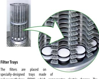
specially-designed trays made of polyoxymethylene (POM) which compensates electric charges. The trays, being self-centring devices, facilitate loading of the weighing pan with the filter, and precise filter positioning in the magazine.
