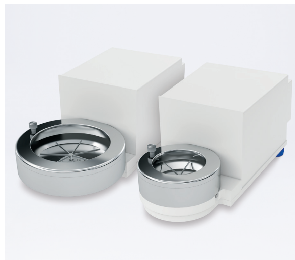
Two different versions of the microbalance enable weighing filters of various diameters.
