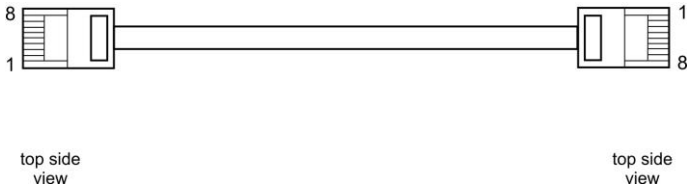
'Mass converter' – ,Ethernet' cable (PT0224)
