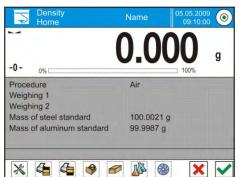
8. Load the pan with steel mass standard, wait for a stable measurement result and
