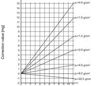
The graph presents correction values for versus the density of weighed load, assumption that air density is constant and equals  $1.2 \text{ kg/m}^3$  is taken.
