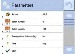
Batch number – identification of controlled products batch Bach quantity – software controls specified number of samples Average tare determining Packages quantity – more than 10
