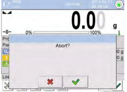
Press button to return to the ongoing control. Press button to abort control and return to **PGC** mode.
