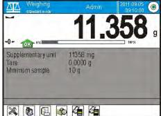
Weight value lower than the MSW value<br/>specified for a particular tare range.Weight value higher than the MSW value<br/>specified for a particular tare range.
