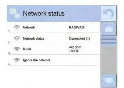
The selected network and connection parameters are saved to balance memory. The program connects to the network in accordance with the memory-saved parameters each time the balance is switched on. To change this, select <Forget network> option. Given network gets disconnected.
