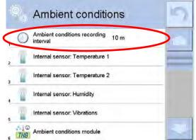
By default the interval is set to 10 min, this value may range between 1 min - 60 min. Record analysis allows the user to select optimal time of the day for the measurements performance, i.e. time when the environmental conditions influence the vibrations the least. Mind that there are places where the most convenient working conditions occur after-hours.
