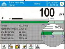
**Caution:** The checkweighing and dosing functions can operate simultaneously in the parts counting mode. In such case the dosing tolerance is controlled by Min and Max thresholds of the checkweighing function.
