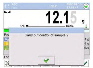
Press 💙 button to confirm. The text and max permissible errors quantity get updated. Upon completed control of sample 2, the software generates control summary. Report on performed control may be printed on a balance-connected printer.
