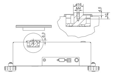
Due to the module high measuring accuracy, it is recommended to install it inside customer's instrument (e.g. in a draft shield) in order to reduce the influence of ambient conditions on the measurement result.
