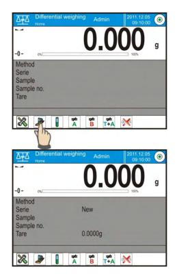
Upon selecting a series, press one of the following buttons determining how the differential weighing is to be carried out:
