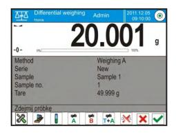
Unload the weighing pan and press <  $\checkmark$  > button.
