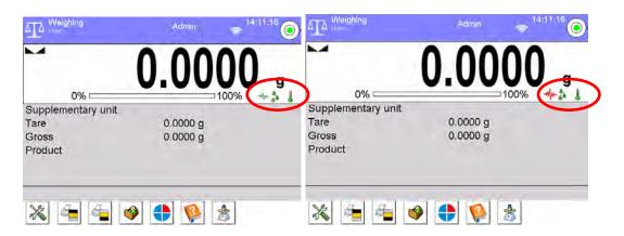
Vibrations are signalled by a respective pictogram displayed in the weighing result window.
