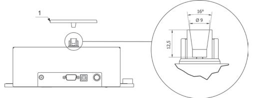
CAUTION: in order to avoid any problems, the used supplementary pan has to weigh about 103g (standard weighing pan, delivered with the weighing module, is 103g).
