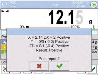
Press button to print report using connected printer. Press button to return to **PGC>** mode settings without printing the report.
