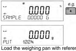
Load the weighing pan with reference sample (which presents 100%). When the indication is stable (
