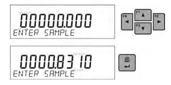
• The software automatically enters <**PARTS COUNTING**> working mode and the weighing instrument displays quantity of single parts (**prts**), and in the bottom line - single part mass value (if such option is selected for <**INFORM.**> function).
