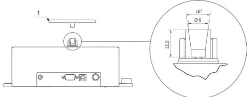
Caution: in order to avoid any problems, the used supplementary pan has to weigh about 103g (standard weighing pan, delivered with a weighing module, is 103g).
