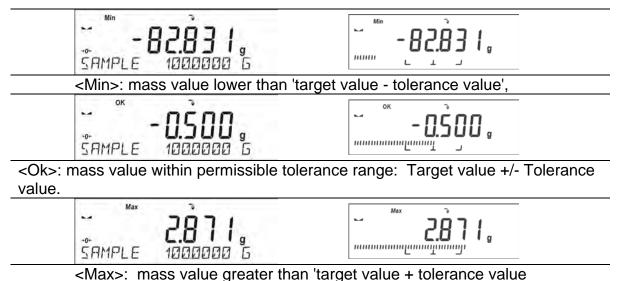
Due to the limited capabilities of LCD display, these symbols do not accurately reflect thresholds settings and target mass, but are meant to visualize settings as a help for operator-balance operation.
