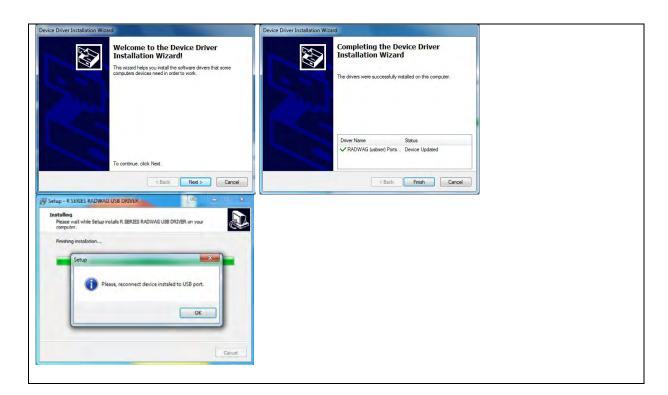
2. Having completed driver installation, connect the module to a computer, use maximum 1.8-meter long USB A/B cable (if the balance is already connected, disconnect it, next reconnect using USB cable).
