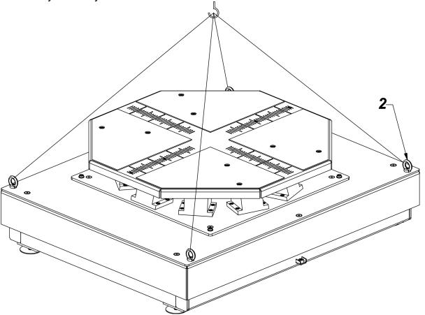
• Upon locating the mass comparator in the place of use, unscrew the screws with eyelets (1), (2) and (3).
