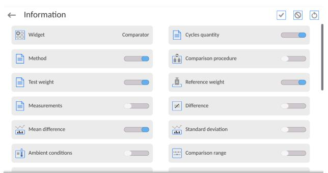
You can quickly change selections of information to be displayed using keys in the top right corner of the screen.
