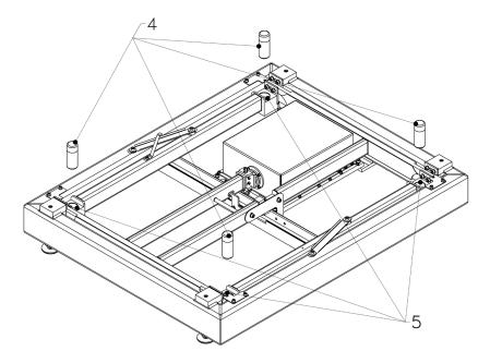
4. Disassemble transport lock by undoing screws and removing fixing washers (6).
