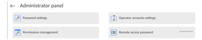
The mass comparator can be accessed remotely using connection to the local Internet network that a computer is connected to. In this respect **VNC Viewer** application can be used. A default password set in the program is a sequence of the following characters: *radwag1234*. If you do not wish to use the default password, you must set your unique access password in the aforesaid parameter.
