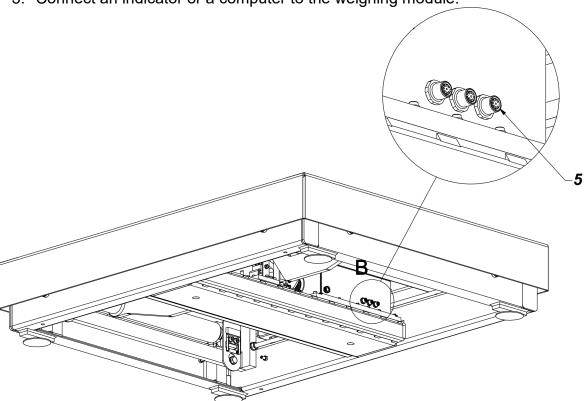
4. Disassemble transport interlocks.
