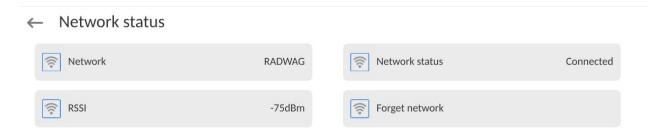
The selected network and connection parameters are remembered by the program and called every time you activate the program and connect to the network. To disable this function, select <Forget network> item. It will terminate the connection to the specific network.
