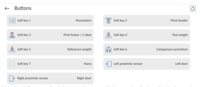
You can define up to 7 quick access buttons, which are to be displayed in the bottom bar. Upon assigning a function to a button a corresponding pictogram is displayed in the bottom navigation bar of the home screen. Each working mode features customized set of buttons. For complete buttons list, read Annex B. These are so called quick access buttons for triggering the most often performed operations.
