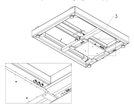
3.Install weighing pan receivers (4), fit them into lever seats (5).
