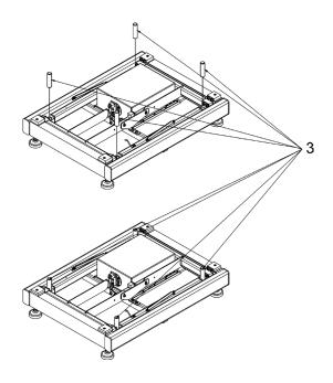
4. Disassemble transport lock by undoing screws and removing fixing washers.
