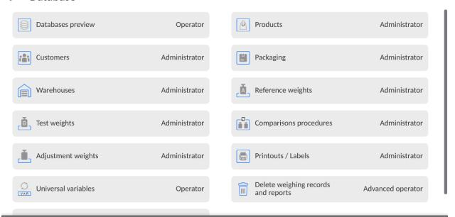
Default mass comparator settings allow the operator logged as **Administrator** to change settings in particular databases. Depending on requirements, these permission levels can be modified.
