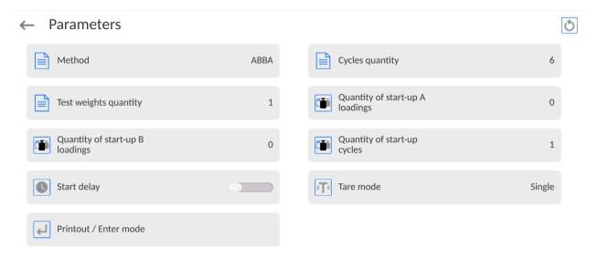
To change the type of weight calibration method, press < Method> key and select the desired method:
