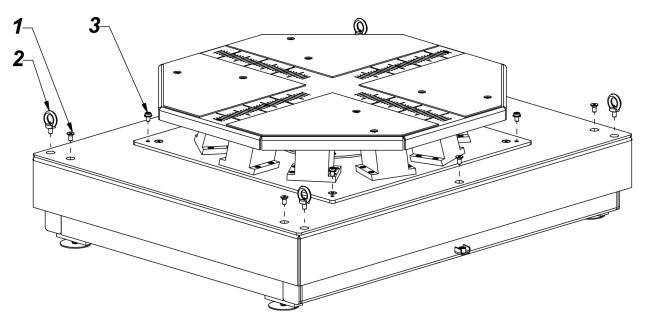
2. Replace the screws (3) with screws with eyelets (2) and using hoist cords disassemble the weighing pan plate (4).
