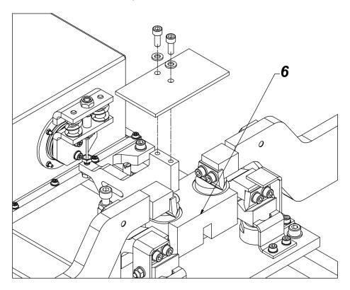
5. Set the bumpers. Loosen the nuts in all four corners. Unscrew the screws and set 1 mm gap. Tighten the nuts.
