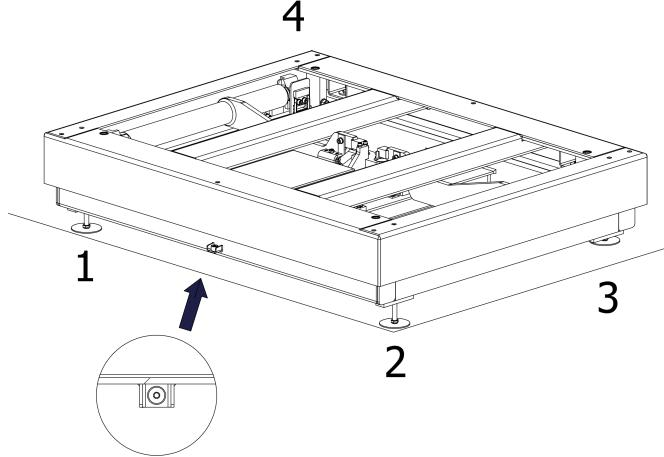
Level the platform using feet no. 1, 2 and 4 until the air bubble takes central position.
