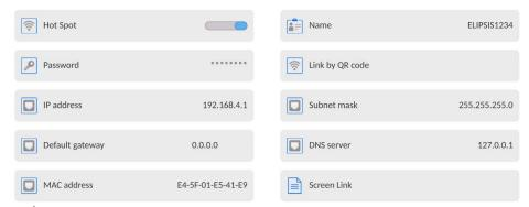
4. From now on, the Hot Spot service will be active and the subnet will be detected by other smartphone devices as the subnet under the aforesaid name, and it will be possible to connect to it via the password.
