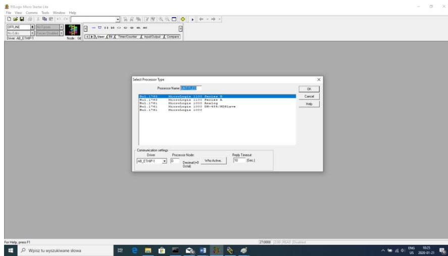
Confirm your choice and go to the project window. Next, configure the communication interface of the controller. To do that, select CHANNEL CONFIGURATION>CHANNEL 1 in the project tree.
