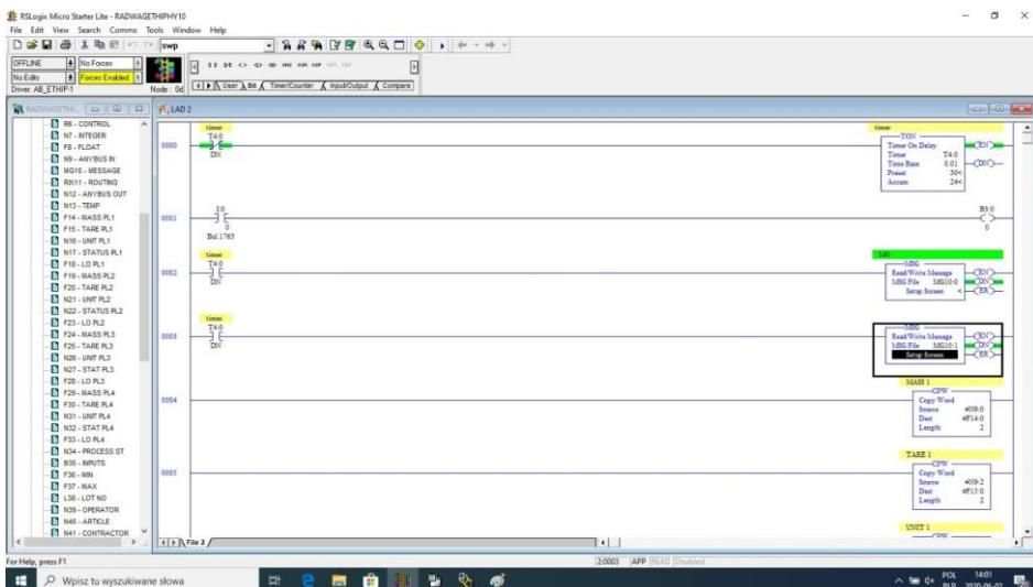
Now you can upload program to the controller and run it. Upon connecting to the PLC (online) in the N9 file it is possible to carry out data readout, the MSG function should not return any errors.
