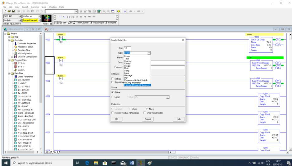
Add also two files of INTEGER type to store data read from the scale and data sent to the scale. In the example two files were created: ANYBUS IN (N9), 120 bytes, and ANYBUS OUT (N12), 120 bytes.
