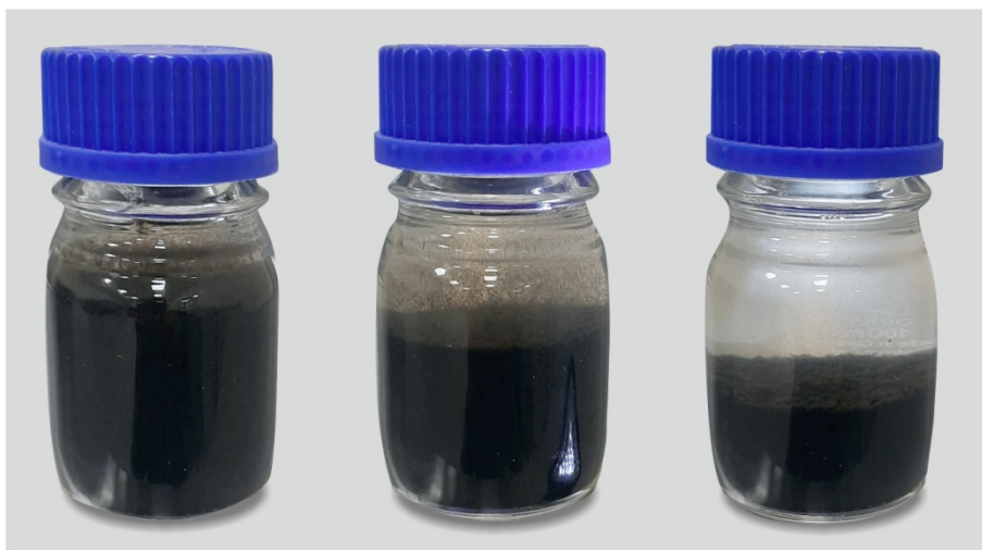
Figure 11. Wastewater sludge sedimentation
