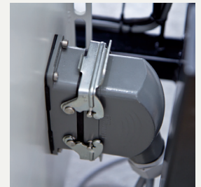
Quick coupling allowing easy detachment of conveyors
