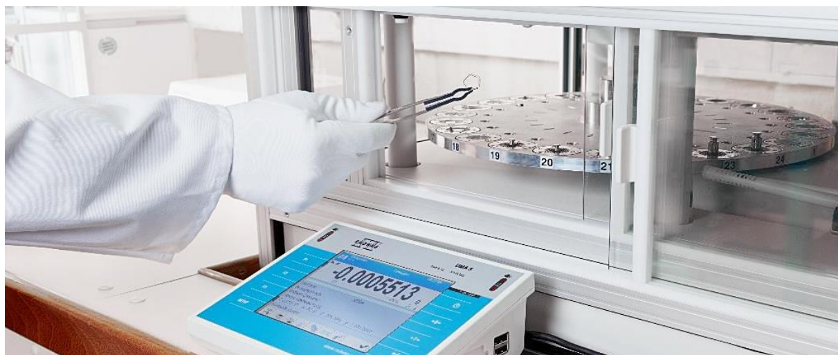
Radwag UMA 5: electric compensation range: 1 mg – 5 g, readability: 0.1 µg
