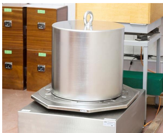
Automatic mass comparator – HRP 500.4Y.KO, d = 0.5 \text{ g} , electric compensation range: 0 \text{ mg} - + 510 \text{ g}
