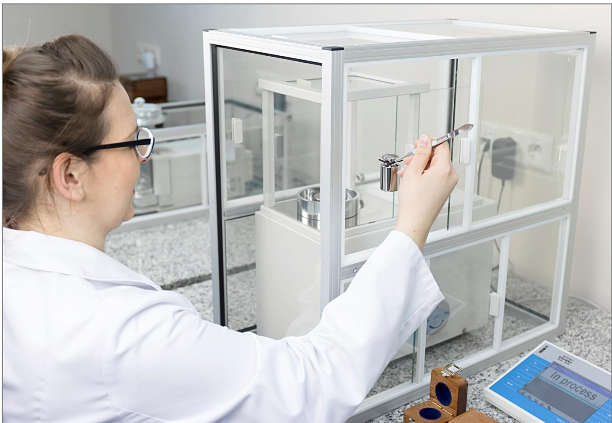
Manual comparison process – mass comparator equipped with an anti-draft shield
