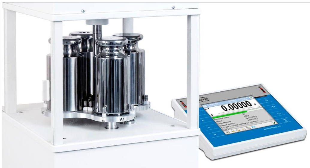
AK-5000 mass comparator, d=0.01 mg Maximum capacity: 5.05 kg, electric compensation range: - 10 g - + 50 g Internal supplementary weights, semi-automatic operation Calibration range: 1 kg – 5 kg
