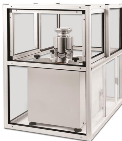
APP 30.4Y.KO mass comparator, d=1 mg, internal supplementary weights, adjustment using external mass standard
