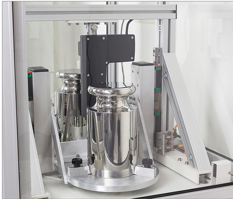
AKM 20-2/20.1 mass comparator, d = 0.1 \text{ mg}
