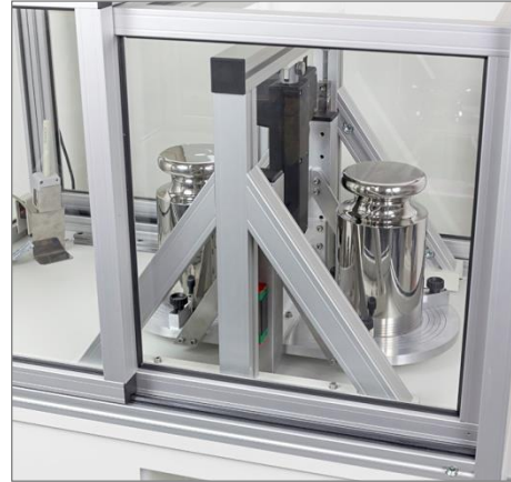
Automatic calibration of 20 kg test weight
