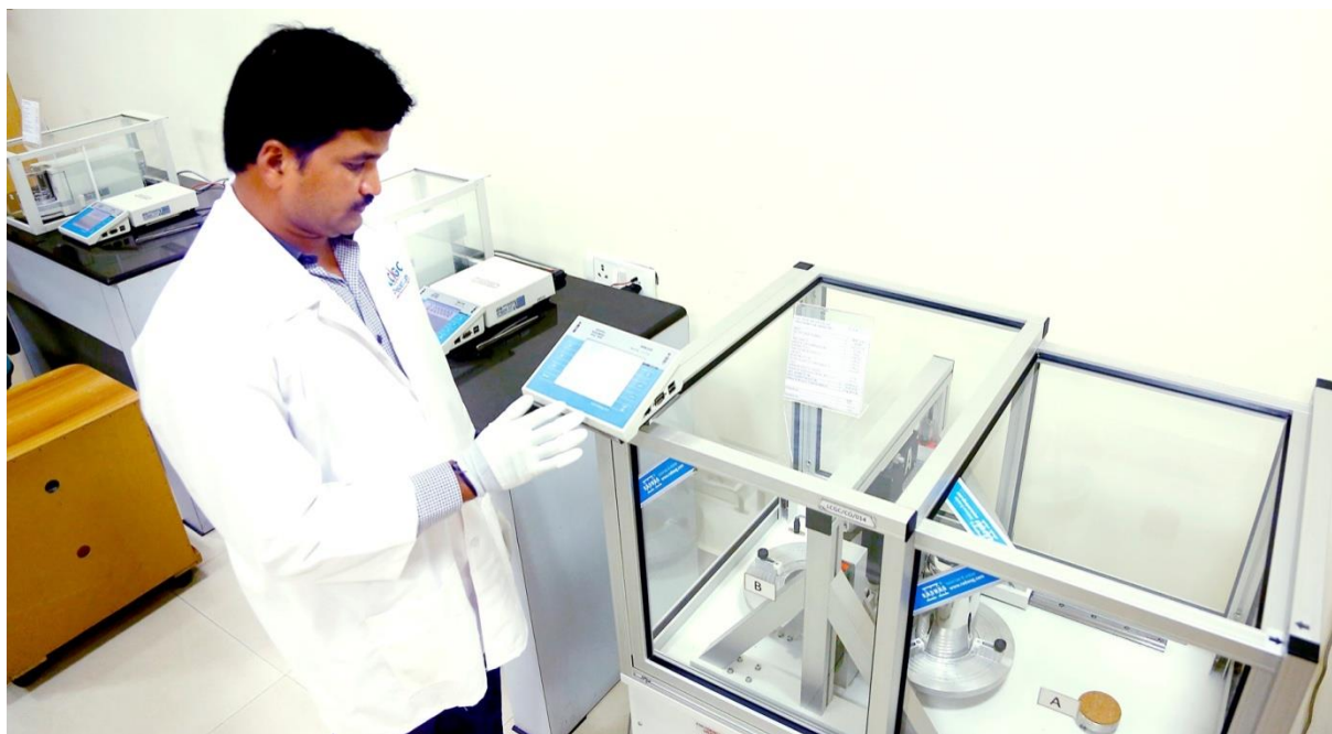
AKM series mass comparator in the course of operation
