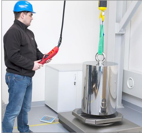
Calibration of 200 kg test weight using self-centring weighing pan
