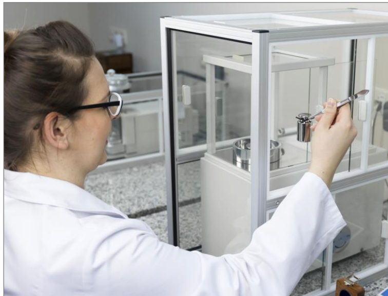
WAY 500.4Y.KO - manual mass comparator, d = 10 \text{ } \mu\text{g}
