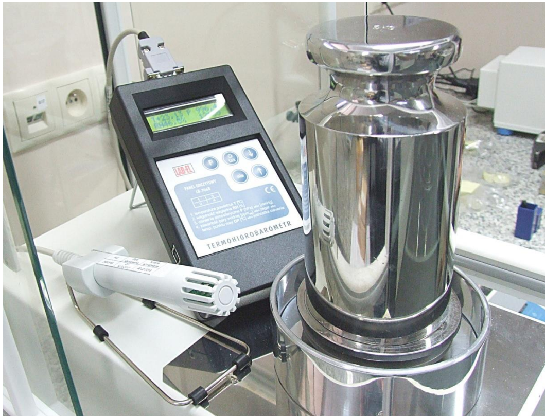
Measurement of temperature, humidity and atmospheric pressure in the course of comparison
