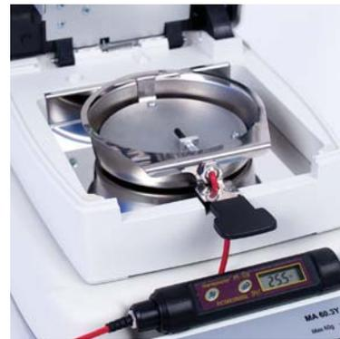
Graduating drying temperature means comparing and correcting indications of moisture analyzer thermometer. The correction is referred to indications of control thermometer, three measuring points are used for comparison. During the test, the control thermometer replaces a weighing pan.
