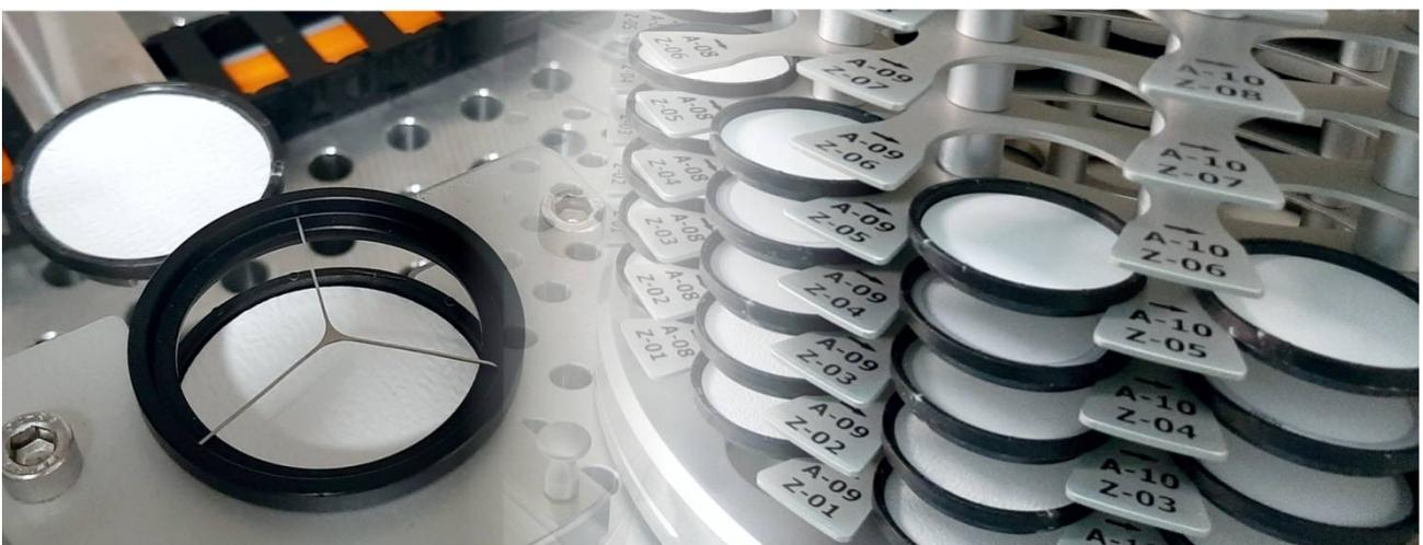
**Figure 54. RB 2.5Y automatic unit – mass standard and filter magazine**
