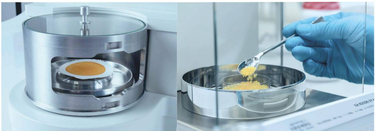
**Figure 13. Testing changes to filter mass after filtering (wastewater treatment plant), measuring the amount of substance (pharmacy)**
