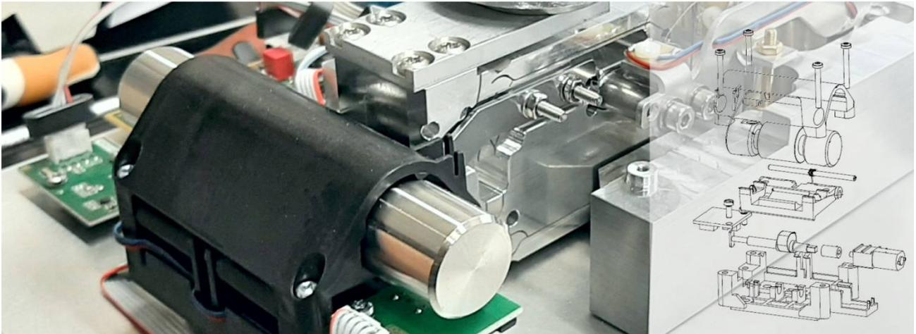
**Figure 47. PS balance adjustment mechanism in the balance with a monolithic measuring unit**
