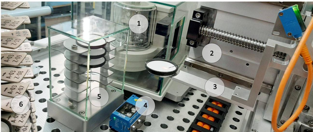
**Figure 35. Filter verification and weighing - RB 2.4Y robotic unit**
