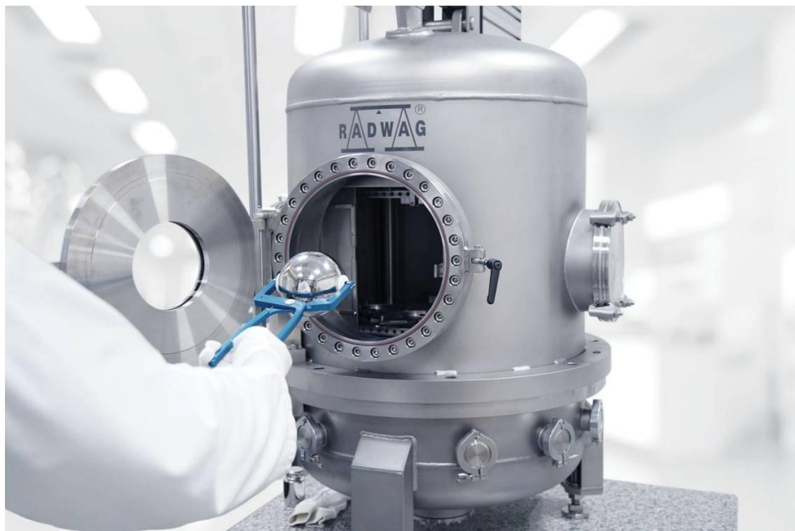
**Figure 3. AVK 1000.5Y vacuum comparator**
