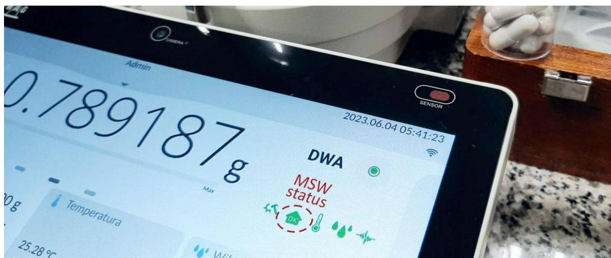
**Figure 14. MYA 5.5Y microbalance with an active MSW function**
