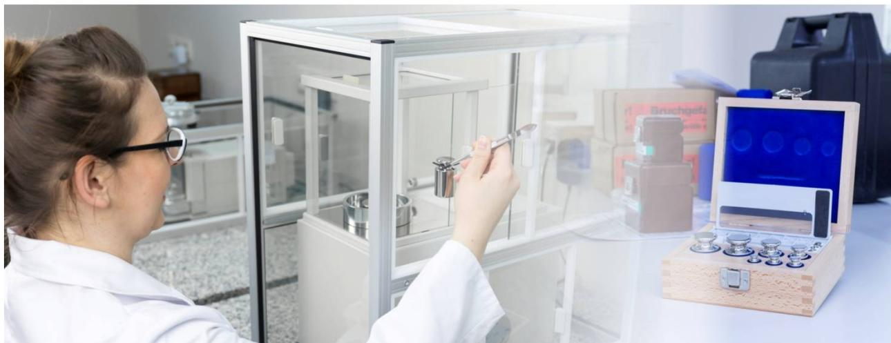
**Figure 5. Manual WAY mass comparator**
