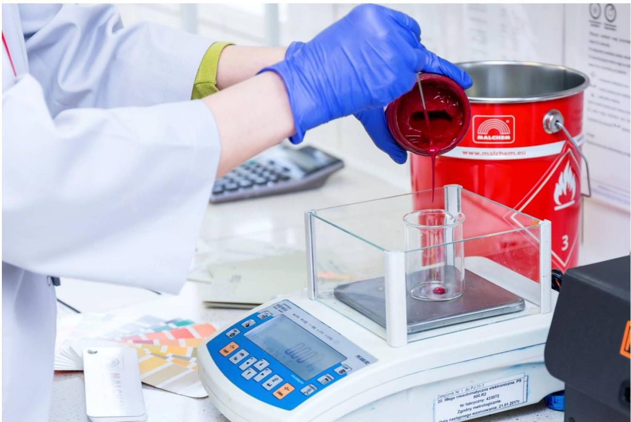
**Figure 10. PS 1000.R2 balance – measuring paint and lacquer mass**
