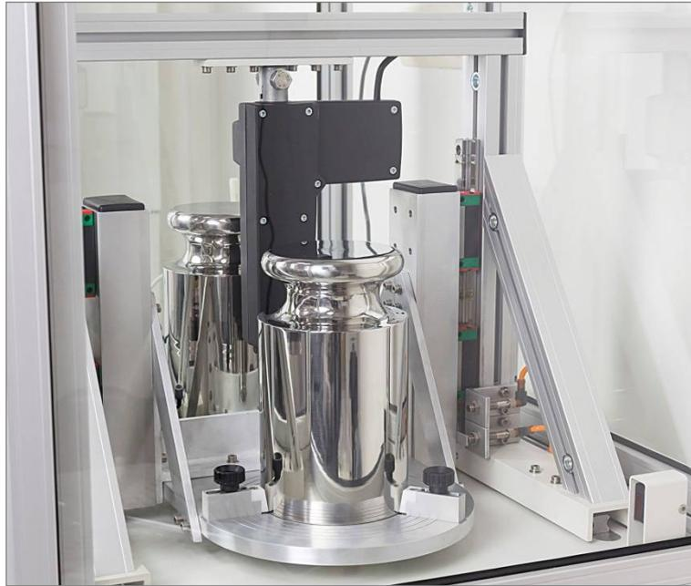
**Figure 2. AKM comparator 2.20.5Y,d= 0,1 mg**
