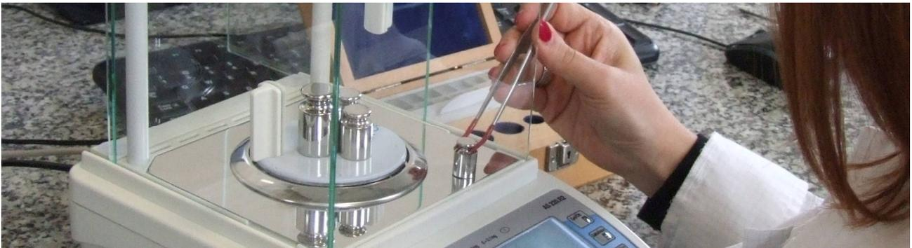
**Figure 11. Quality Control Department – AS 220.R2 balance, evaluation of correct values**
